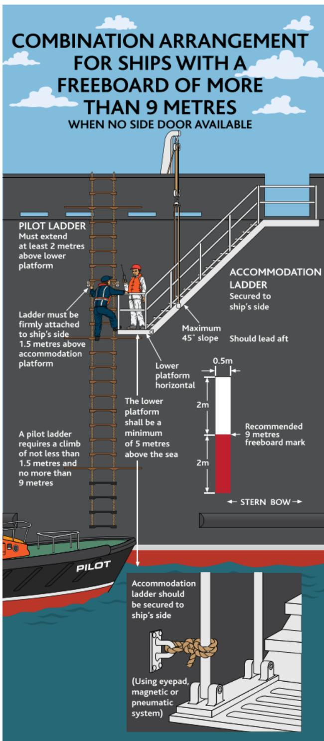
**NOTE:** – The pilot ladder is required to be rigged two (2) metres above the water.
