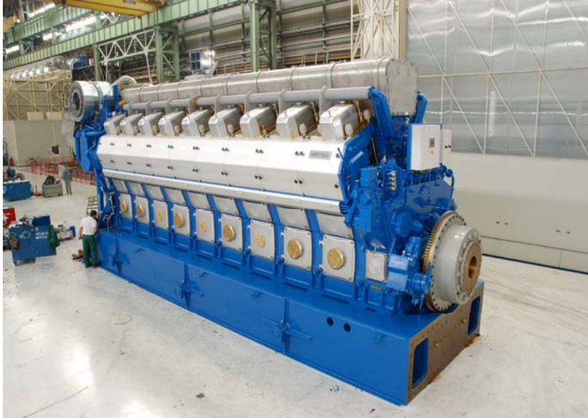
50 bore DF Engine, 950 KW/Cylinder
