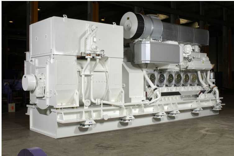
26 bore Engine, 340 KW/Cylinder
