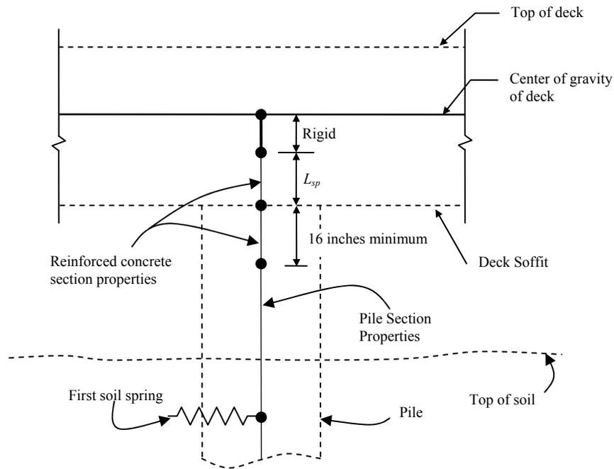
**Figure 1-1: Modeling of Pile-to-Deck Connection (Not-to-Scale)**
