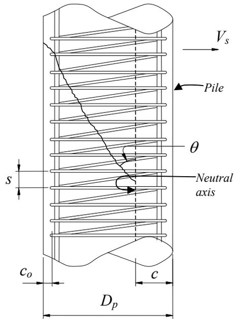
Figure 1-5: Pile Transverse Reinforcement Shear Strength Component
