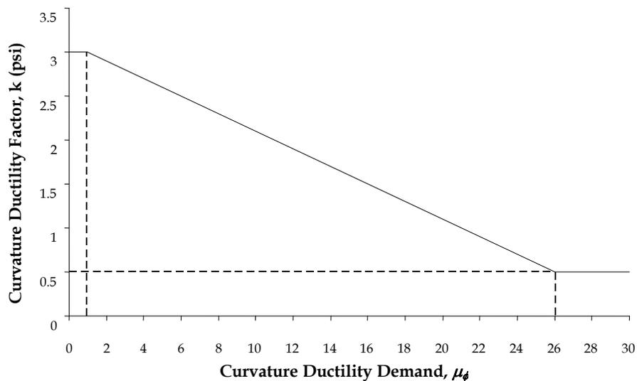
**Figure 1-4: Curvature Ductility Factor Versus Curvature Ductility Demand**
