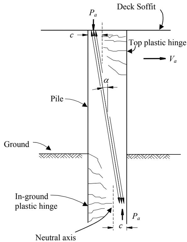
Figure 1-6: Pile Axial Force Shear Strength Component
