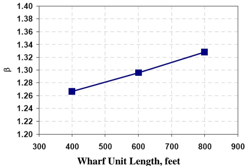
**Figure 1-7:  $\beta$  Versus Wharf Unit Length**
