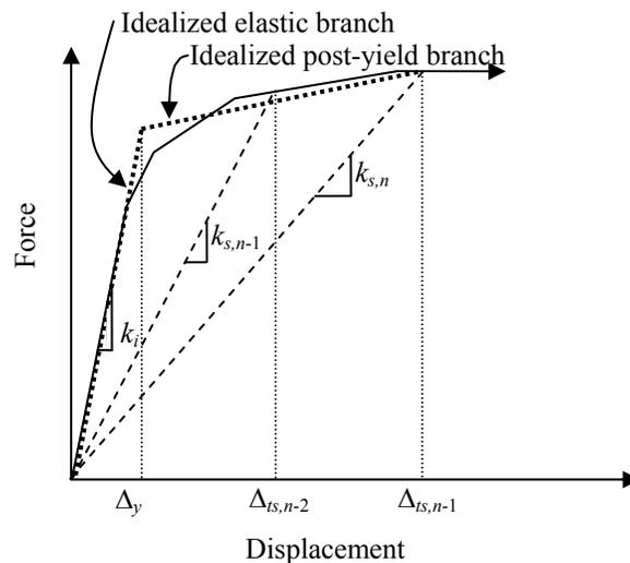
**Figure 1-3: Force-displacement Curve**
